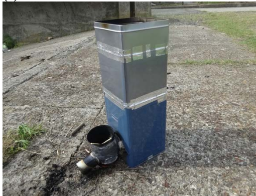
Fig. 7 Rocket heater (a) Outside view of heater, (b) Mechanism of heating
